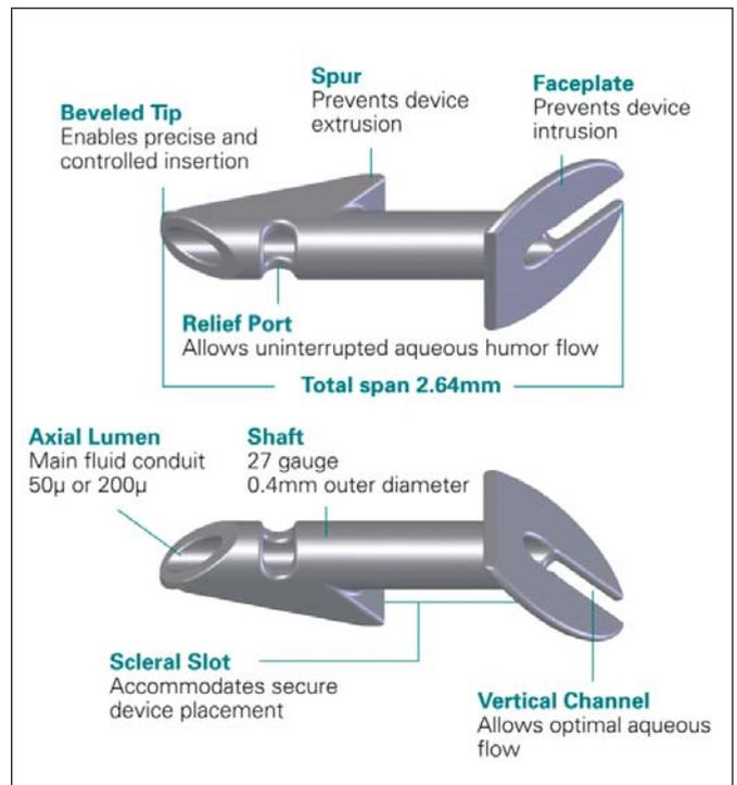
Figure 1. The EX-PRESS Glaucoma Filtration Device.
