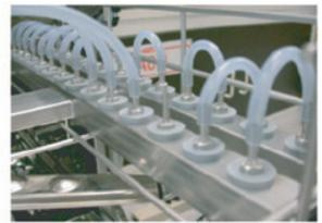
**Step Seven:** Plug off any unused injector nozzle with silicone tubing.
