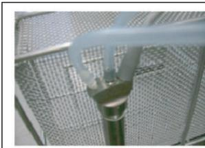
**Step Five:** Using the Auto Wash Kit, secure the handpiece to the wire mesh basket using the small gauge wire and connect the handpiece with the "Y" adapter assembly as shown.
