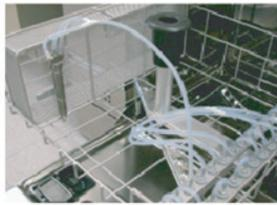
**Step Six:** Place wire basket with handpiece in multi-purpose injector rack and connect the "Y" adapter assembly to the 4 mm diameter injector nozzle as shown.
